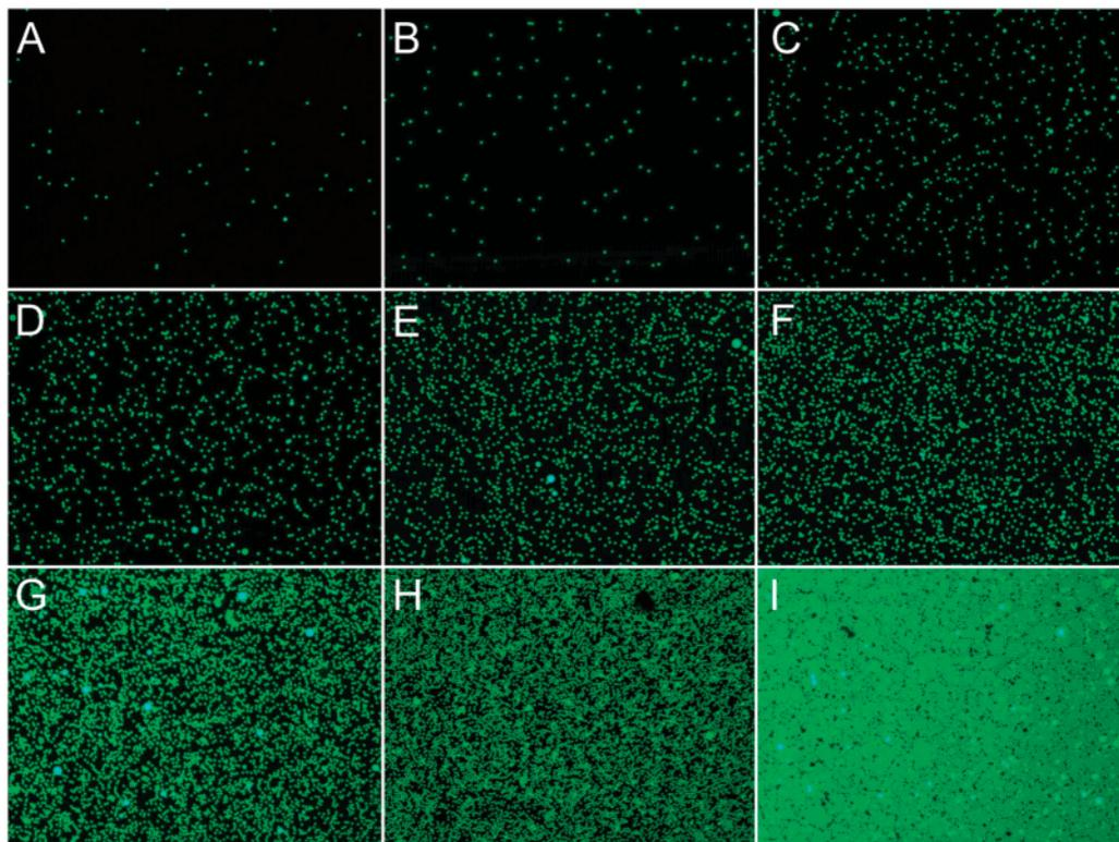
**Figure 2.** Varying particle concentration and settling time produced surfaces with a wide range of densities of 2 micron particles (green), functionalized with the protein streptavidin. Specific conditions for the preparation of each surface, samples A–I, and the resulting surface coverages and particle spacings are reported in Table 1.
